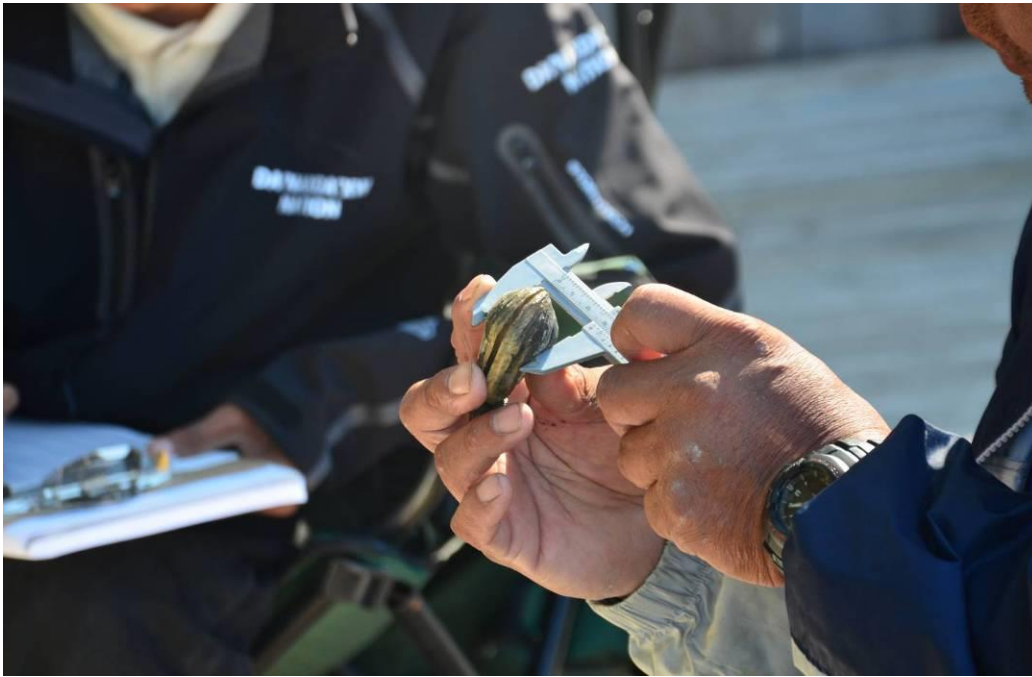
Obtaining a thickness measurement using calipers.
